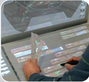
In Strip'TIC, controller actions such as strip moves and pen input are instantaneously known from the system (even outside the stripboard, pen input still works).
